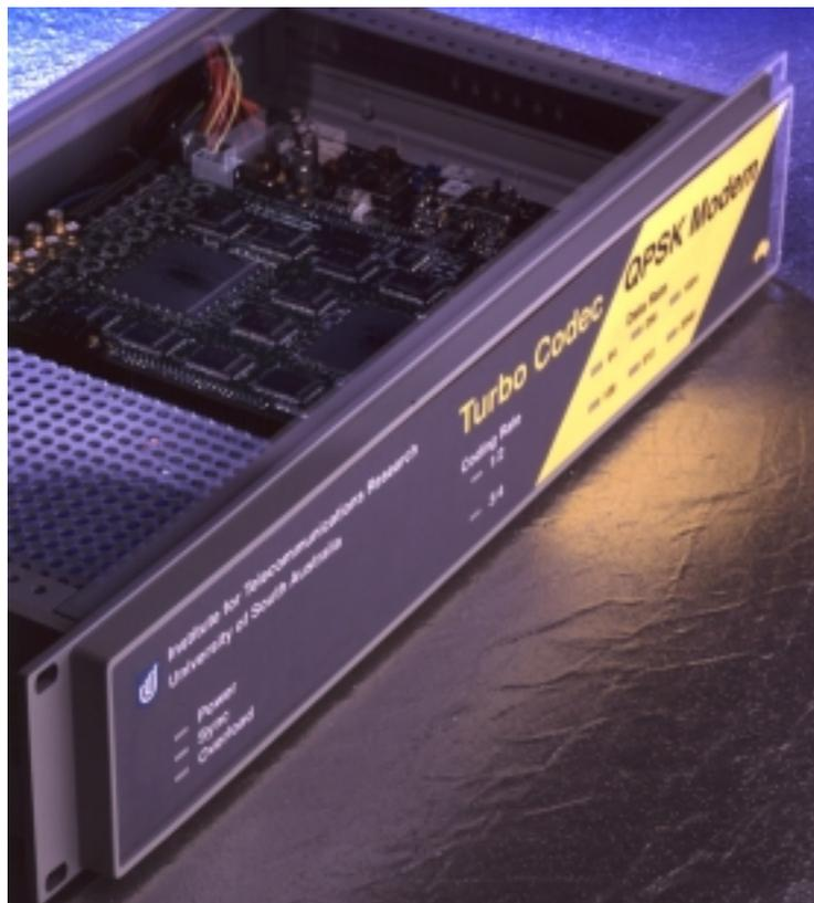
Figure 5: *Turbo Codec – QPSK Modem*
