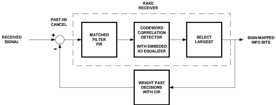
Figure 8. Rake receiver with ISI/ICI equalizer
