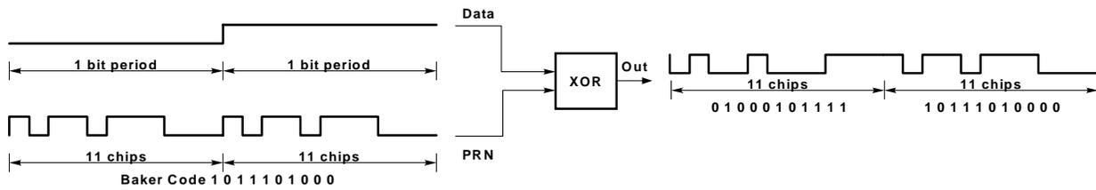
Figure 1. Digital Modulation of Data with PRN sequence
