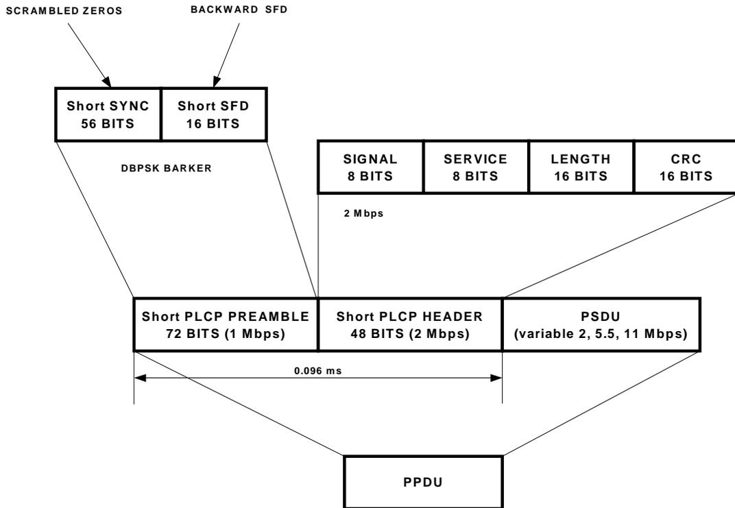
Figure 6. Short PLCP PDU format.
