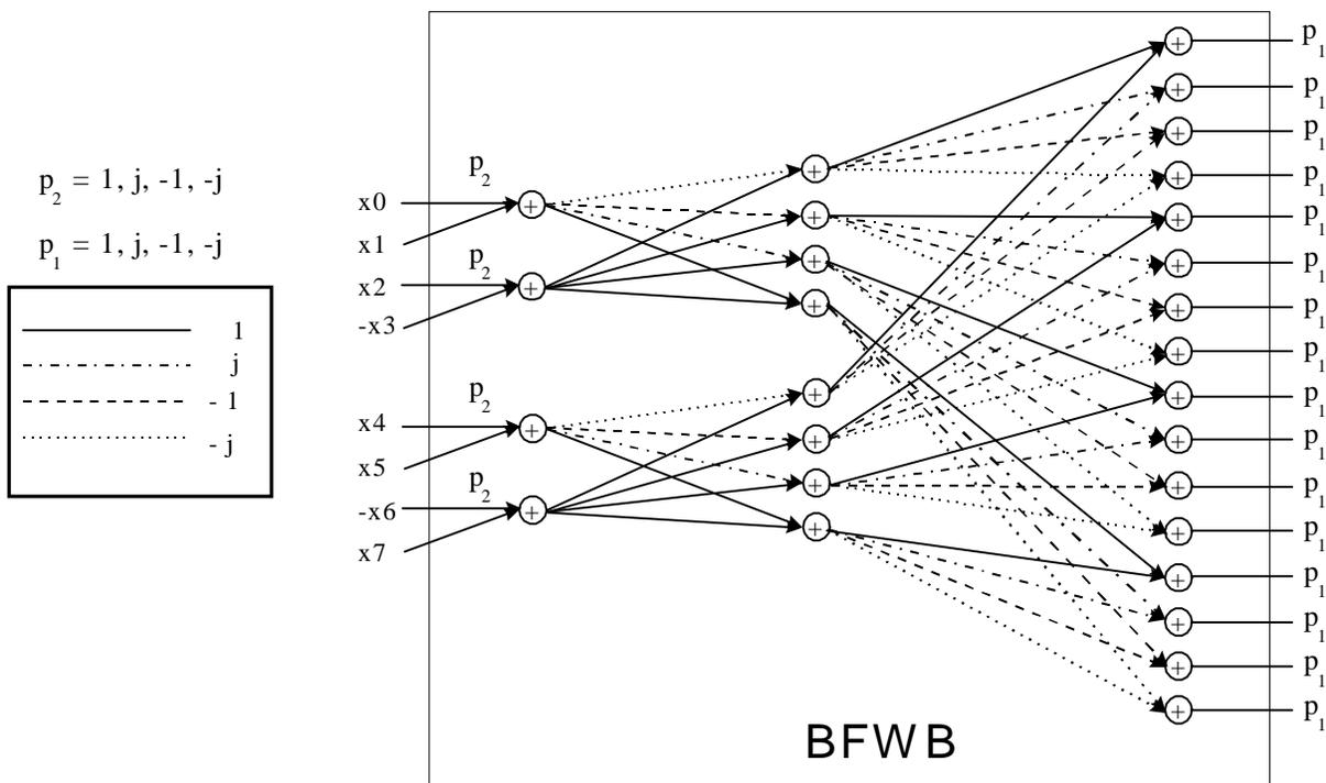
Figure 2. Basic Fast Walsh Transform Block (BFWB).
