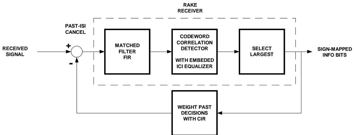
Figure 8. Rake receiver with ISI/ICI equalizer
