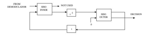
Figure 7. Decoder for SCCC.
