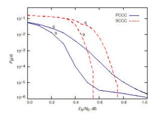
Figure 10. Comparison between PCCC and SCCC techniques.
