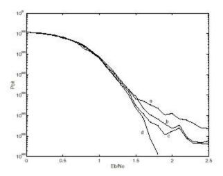
Figure 4. Convergence of "constellation" interleaver for PCCC
