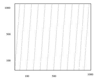
figure 8. Interleaver for SCCC
