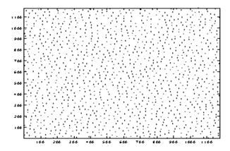
figure 5. Interleaver for PCCC
