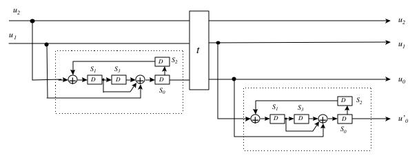
Figure 6. Serial Convolutional Concatenated Encoders
