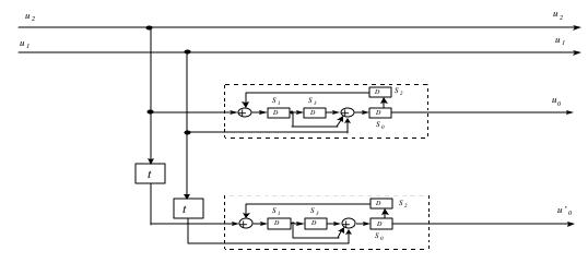
Figure 1. Parallel Convolutional Concatenated Encoders
