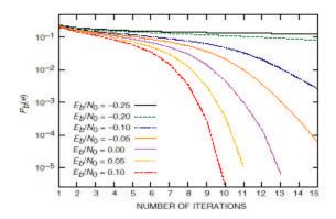
Figure 9. Convergence of iterative decoding for SCCC using ASW-SISO algorithm
