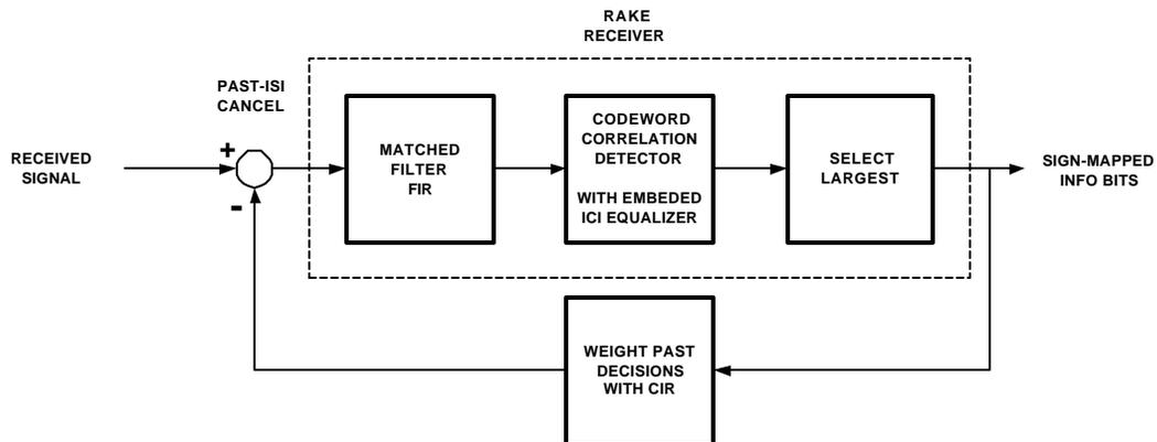
Figure 8. Rake receiver with ISI/ICI equalizer
