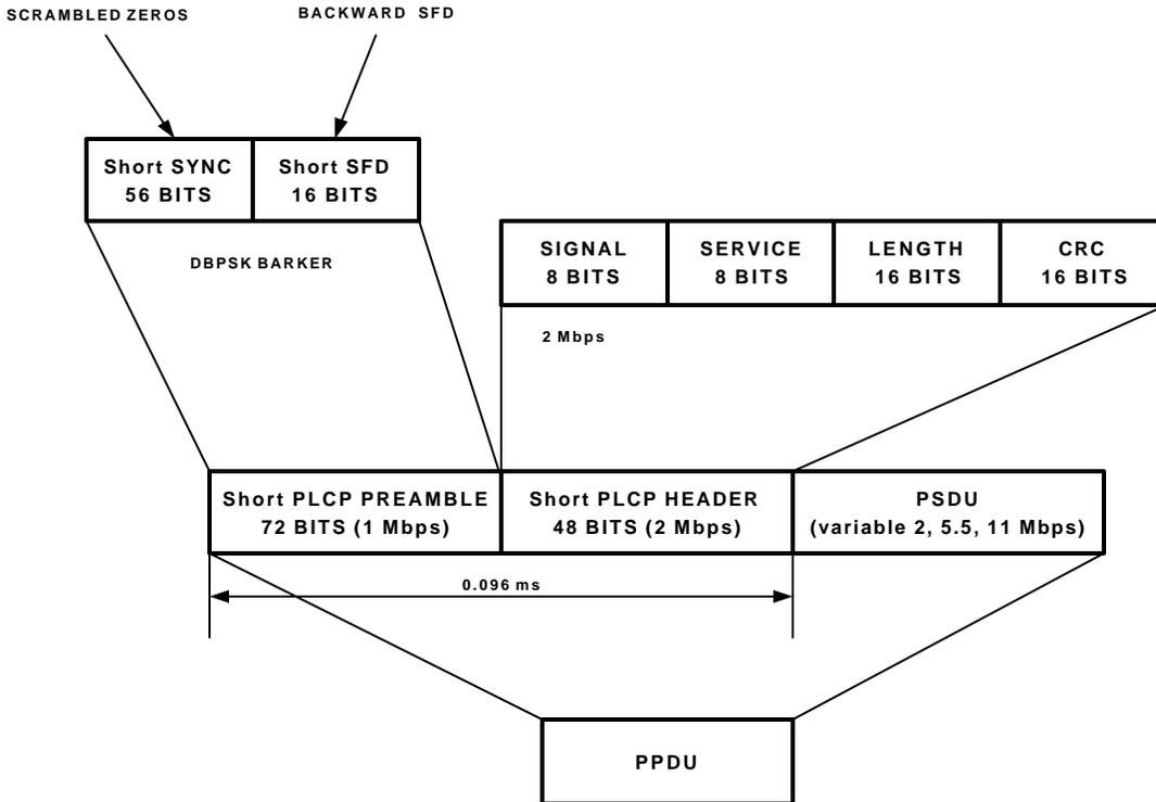
Figure 6. Short PLCP PDU format.
