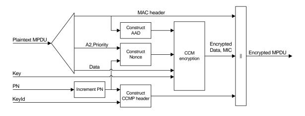
Figure 1. CCMP AES Encapsulation Process
