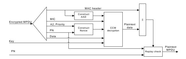
Figure 4. CCMP De-capsulation
